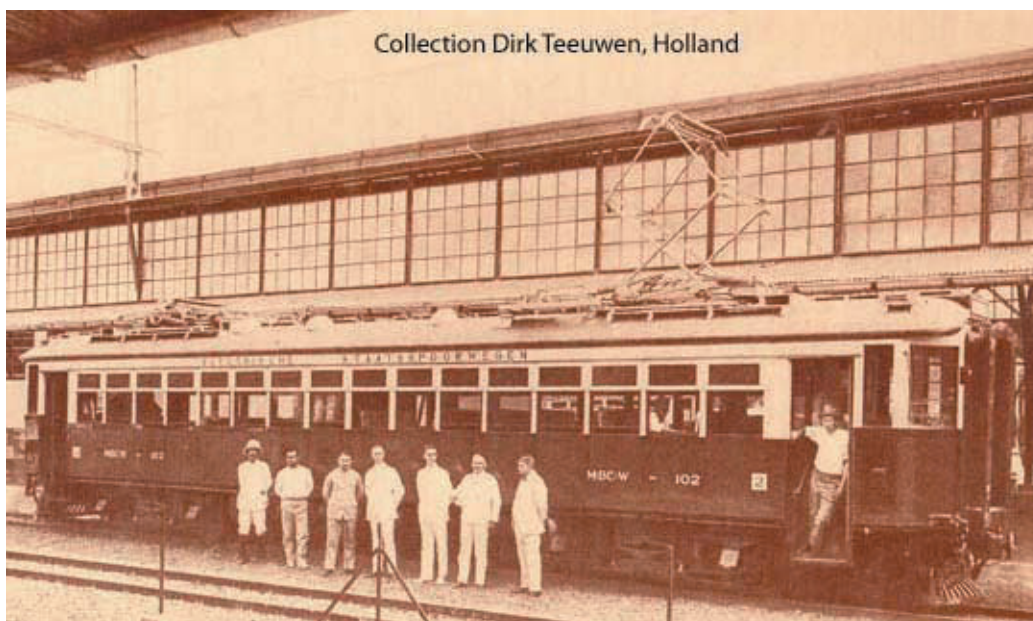
3.6 Electric motor passenger coach meant for urban traffic (2 nd and 3 rd class); Batavia-Jakarta 1924
