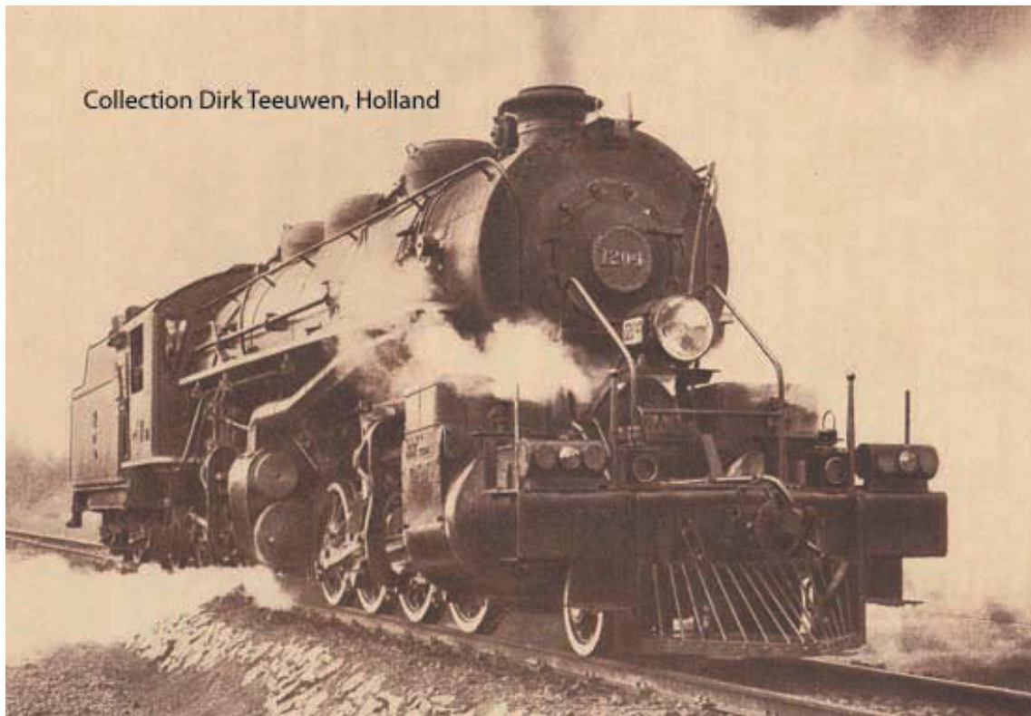
P.1.1 Mallet mountain locomotive, Preanger 1925 Dutch East-India The Mallet Locomotive is a type of articulated locomotive invented by a Swiss engineer named Anatole Mallet (1837-1917). Mallet's original design was a compound locomotive in which the steam is used twice, first in a set of high-pressure cylinders, then in a set of low-pressure cylinders. It is quite easy to find more information on the internet.
